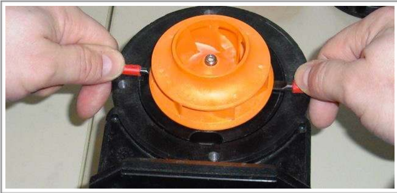
Fig. 2: Loosening of impeller components (rotor unit)
