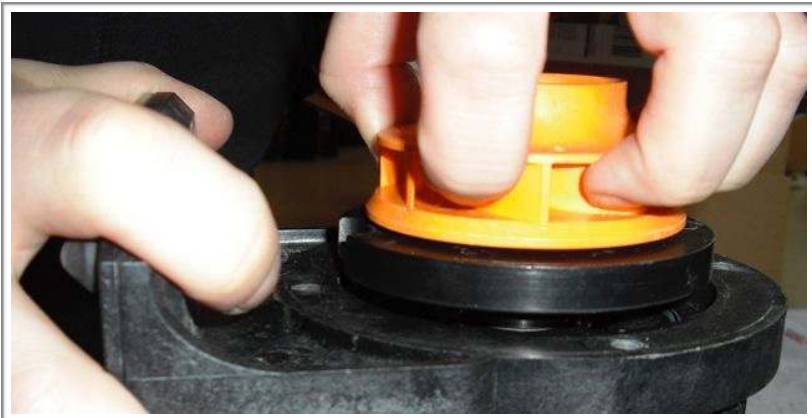
Fig. 3: Disassembly of impeller components (rotor unit)
