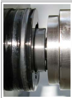
Fig. 4 a/b: Removed impeller component and close-up of bearing (left)
