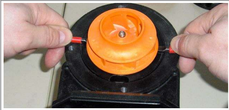
Fig. 6a: Loosening of impeller components
