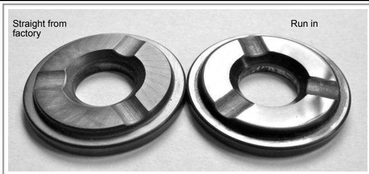
Fig. 2: Bearing straight from factory and following run-in phase
